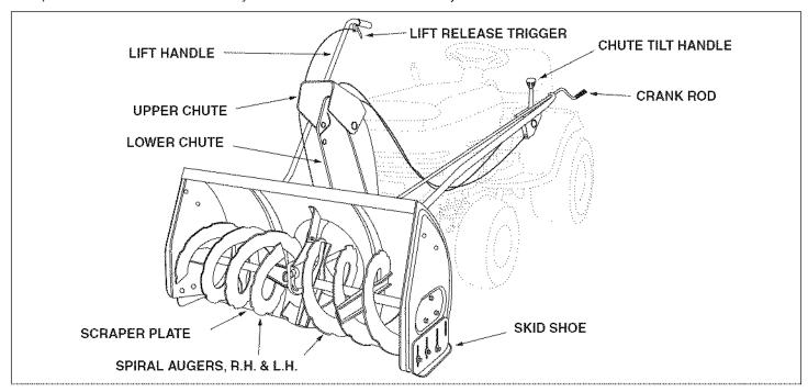
CHUTE TILT HANDLE Pivots the Upper Chute up or down to control the angle and distance of discharge. CRANK ROD Rotates the Lower and Upper Chutes to control the direction of discharge.
